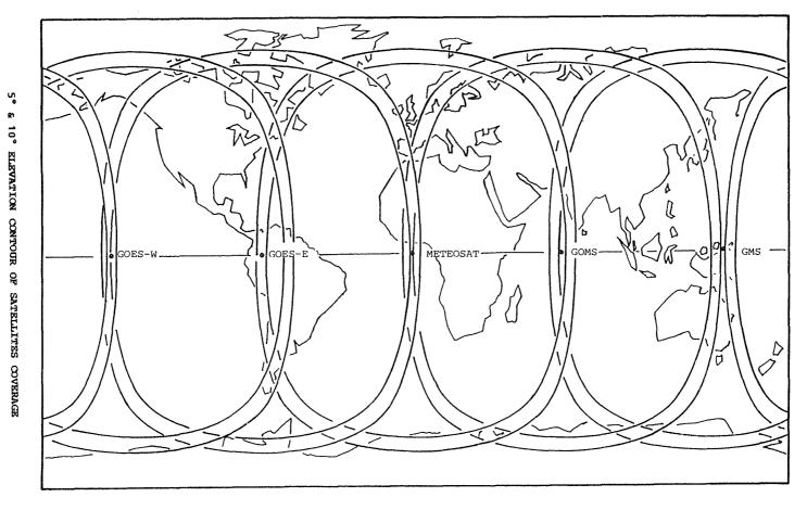
FIG.2 Geostationary meteorological satellite radio footprints (Courtesy CGMS)
