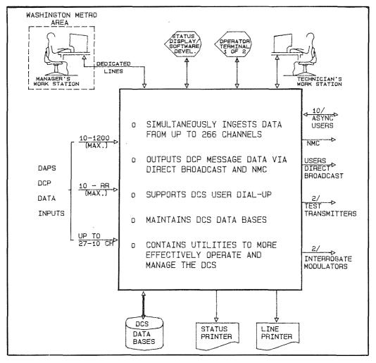
FIG.5 New GOES DCS ground system capabilities
